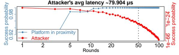
Figure 8: Parameter tuning: the attacker’s success probability  $P_{adv}$  and the legitimate success probability  $P_{legit}$  for different number of rounds  $n$  given a fixed  $k$ .
