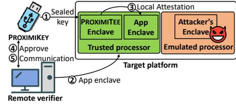
**Figure 9: PROXIMITEE boot-time attestation.** After the boot-time initialization (refer to Figure 10) the PROXIMITEE enclave executes a local attestation with the verifier uploaded application-specific enclave.
