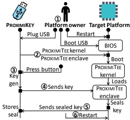
**Figure 10: Boot-time initialization.** The PROXIMiKEY uses a minimal kernel Linux image to boot and load PROXIMiTEE enclave on the target platform and seal a platform specific secret to the PROXIMiKEY memory.
